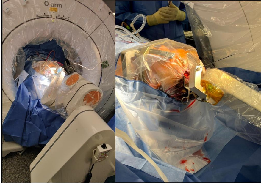
Figure 3. Patient undergoing a sEEG procedure with a Neuromate® stereotactic neurosurgery robot.
